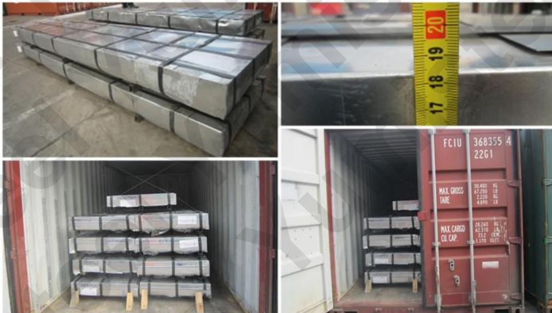
Firstly,PVC film to pack steel roofing sheets,then use mildewproof kraft paper to pack outside and finally use steel box packing.
