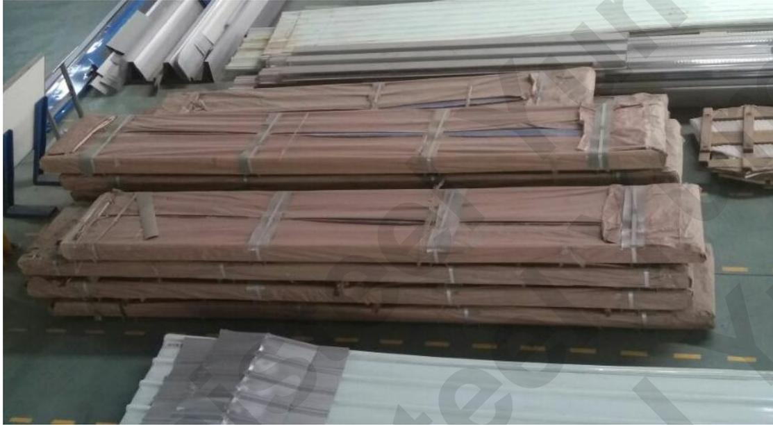
Firstly,PVC film to pack steel roofing sheets,then use mildewproof kraft paper to pack outside.
